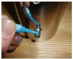
STEP #03 Apply Thread Locker Apply Thread Locker to each set screw per instructions on tube.
