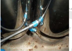
STEP #08 Securing Tips Thread in the 4 bottom set screws until screw touches tailpipe
