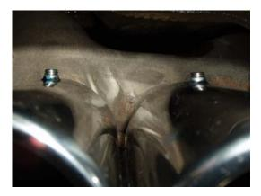
STEP #07 Just a few threads should show after finger tightening.
