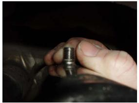
STEP #06 Securing Tips Tighten top set screws with fingers until set screw touches tailpipe
