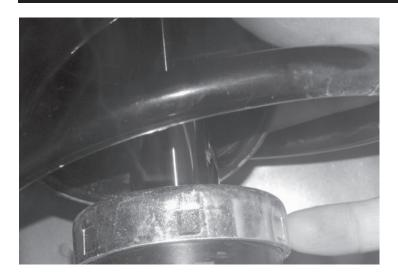
Step#01 (FRONT) Detach the bottom of the dust boot on the front strut.
