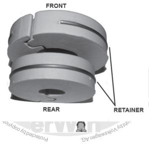
Step#03 Install the retainer on the suspension limiter and slide to the stop at the top of the strut. Repeat for other side.
